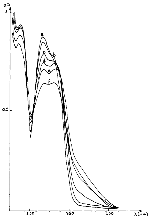
Figure 1. Changes in the UV spectra of polysiloxane 2d upon irradiation for (a) 0, (b) 5, (c) 15, (d) 30, and (e) 45 min and (f) photo-cross-linked film after washing with dichloromethane.
